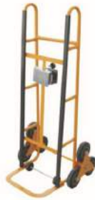
Model No. HT0608 Load Capacity 200 KG Wheel 6.5"X1.75" solid L/W/H(MM) 1355/575/605
